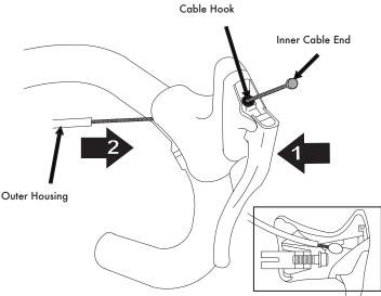
4. Attach the cable to the brake following the brake manufacturer's instructions. Depress the lever a few times to be certain the cable and housing are properly seated before making final adjustments. NOTE: Lubricate the A position if a squeaking noise occurs after a long period of use.
