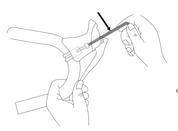
3. Provisionally secure the housing to the handlebar using electrical tape or something similar. With the housing in place on the handlebar cut the housing to the proper length. For the rear brake, be sure to allow enough room for the handlebars to turn all the way to the left and right without pulling on the cable.
